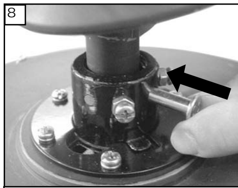
8 Align hole in downrod with hole in yoke and install cross pin.
